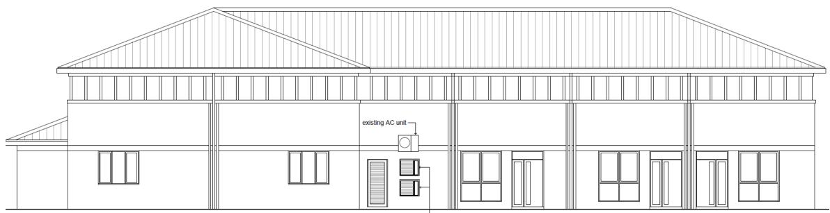
location for 2 No DAIKIN RXM50N2V1B9 condensing units for air conditioning system. Each unit 870mm width X 734mm height
