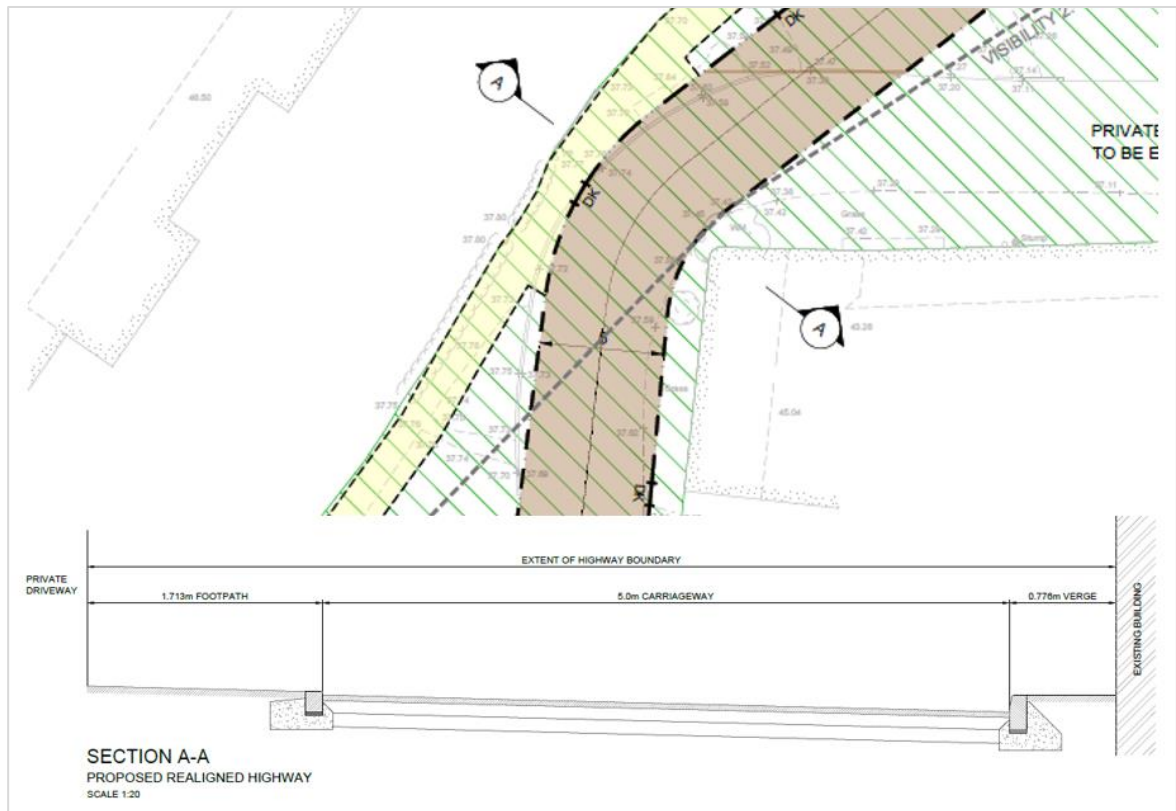
Figure 2: Extract from drawing number 215077-CCL-XX0XX-DR-C-0001 Rev. P05 indicating the pinch point in footway width
