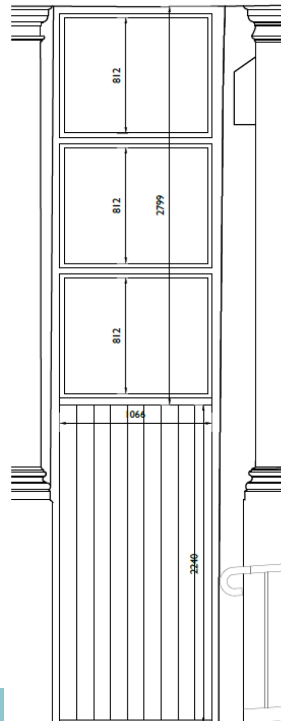
Alleyway Door, DG01 Elevation A-A as Proposed - 1:20 @ A3
