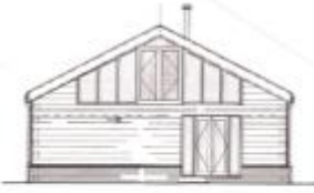
Proposed East Elevation - clearly shows windows behind slats Scale 1:100
