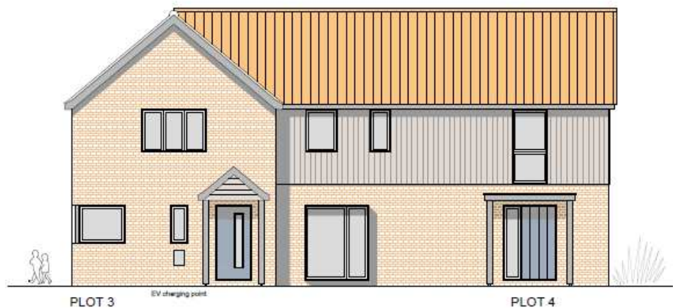
STREET ELEVATION PLOTS 3 & 4 Red multi facing brickwork, red pantries, vertical composite boarding, PPC aluminium composite windows & doors, timber porches
