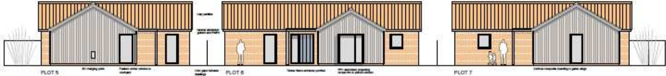
STREET ELEVATION PLOTS 5, 6 & 7 Red multi facing brickwork, vertical composite cladding, red clay pantiles, PPC aluminium composite windows and doors, timber porches
