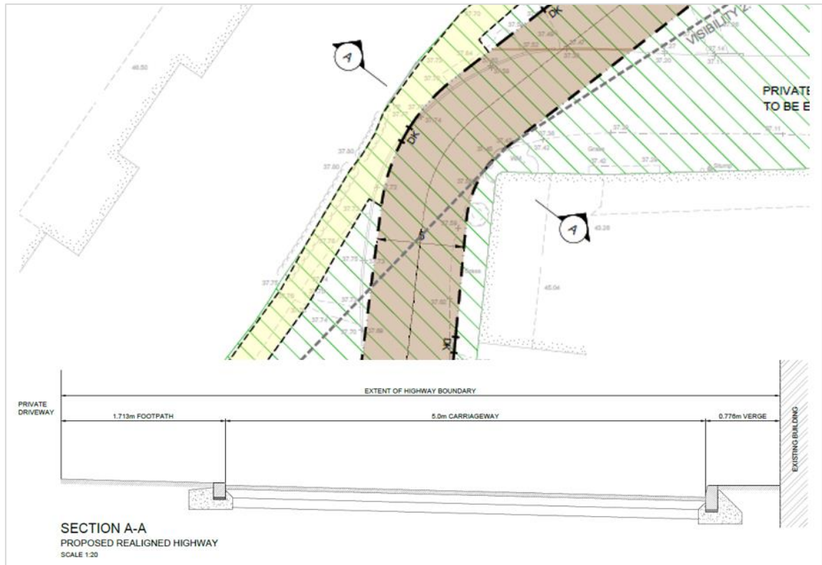
Figure 2: Extract from drawing number 215077-CCL-XX0XX-DR-C-0001 Rev. P05 indicating the pinch point in footway width
