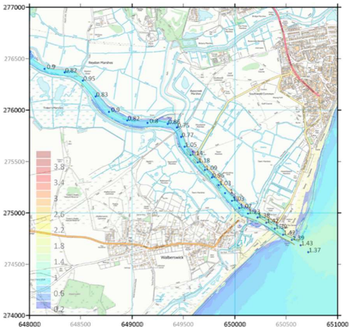
Figure 5-12: Peak flow rates (present-day defences, February 2020 conditions)
