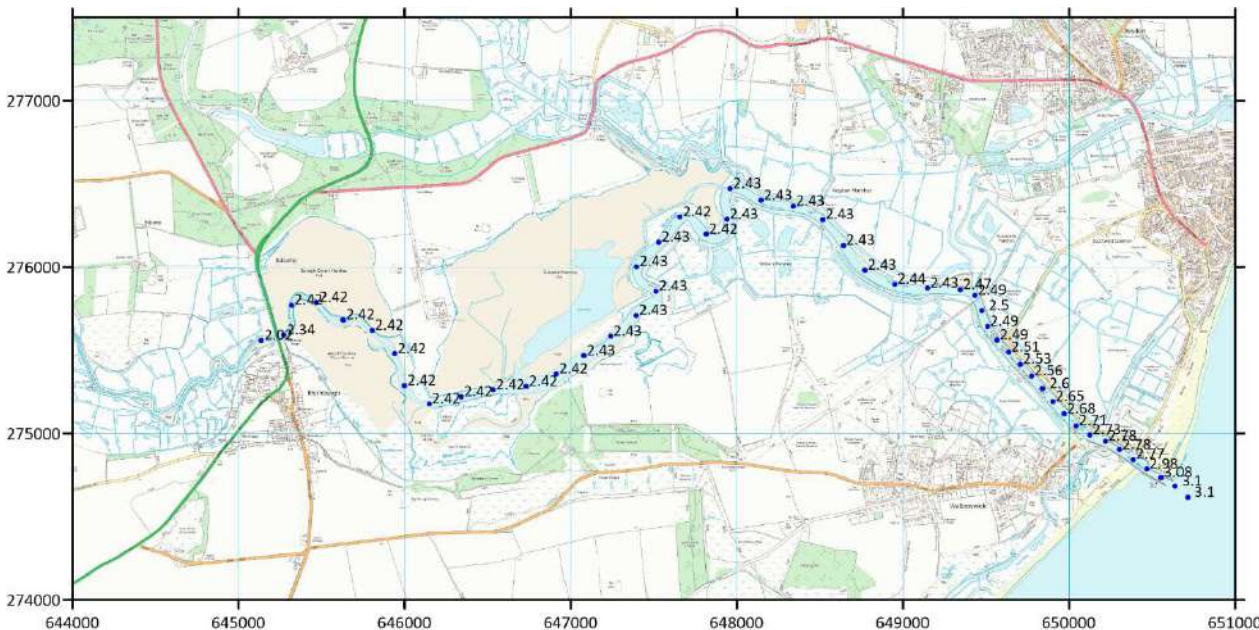
Figure 5-9: Peak flood levels (present-day defences, December 2013 conditions)
