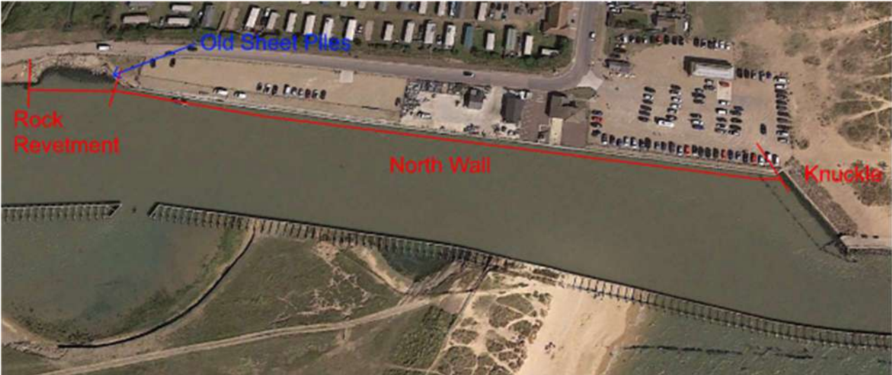
Figure 4-17: Plan of North Wall and Knuckle, showing rock revetment and old sheet piles
