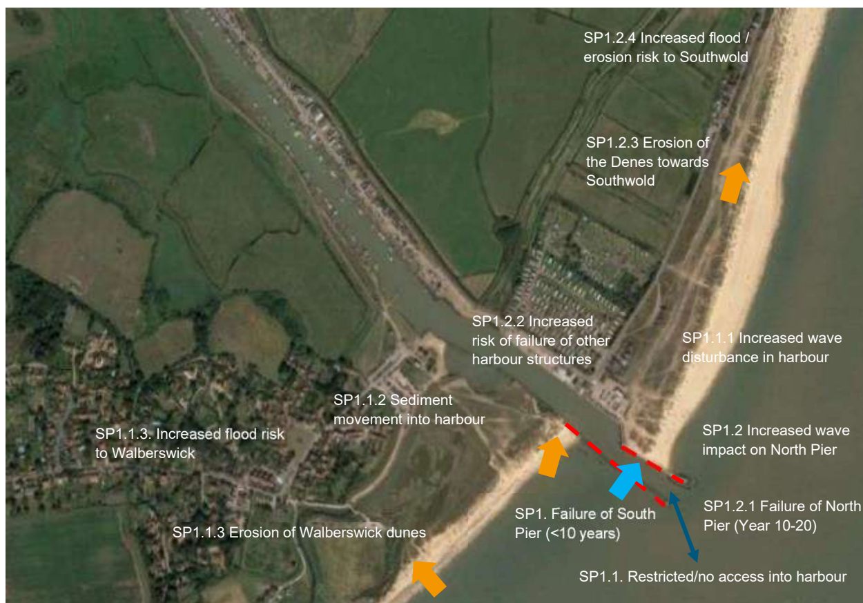
Figure 6-1: Illustration of impacts of Do Nothing scenario for the harbour entrance structures
