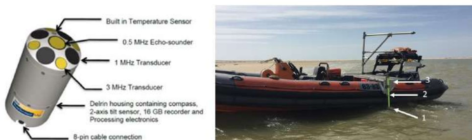
Figure 4.27: Example of vessel-mounted RiverSurveyor M9. Left: M9 graphic and specifications. Right: M9 mounted on the survey vessel, note the submerged ADCP (annotation 1), the vertical attachment pole (annotation 2) and the mounting frame (annotation 3).
