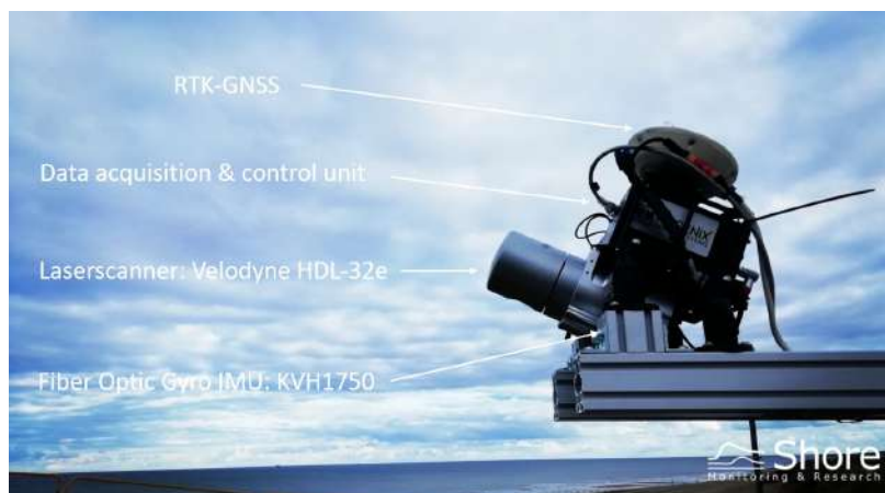
Figure 4.8: Mobile LiDAR system mounted on the survey vehicle. Components indicated in the picture.
