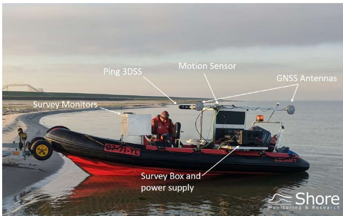
Figure 4.2: Example of SHORE’s 3DSS PingDSP survey system on a tailored RIB. Components indicated in the picture.
