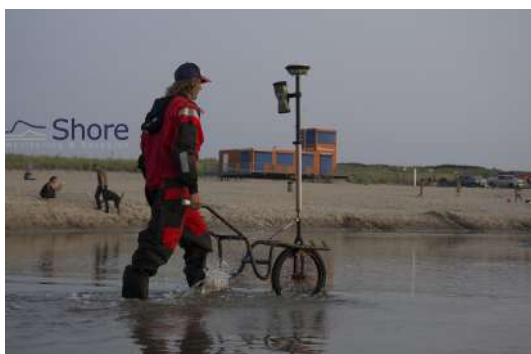
(a) Acquiring height validation data with SHORE's GNSS Carrier.
