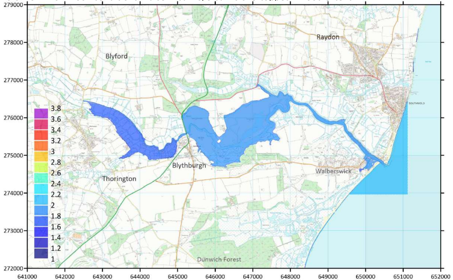
2070 with 0.6m SLR from 2002 conditions: Raise N banks, S banks overtopped – flood extent
