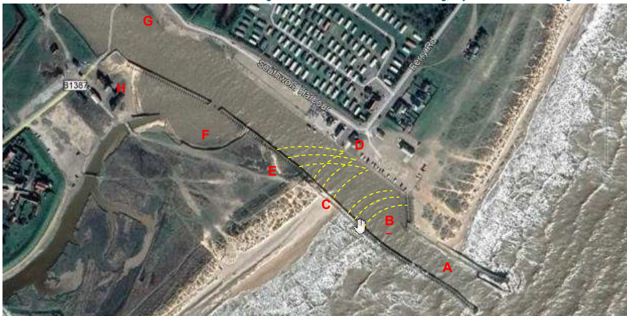
Figure 5-3: Wave behaviour at Southwold Harbour
