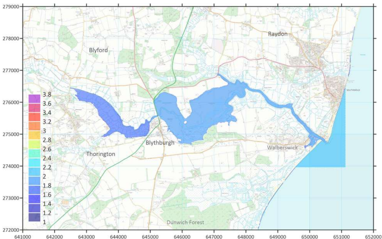
Figure 5-16: Flood extent and depth (present-day defences, Feb 2020 conditions + SLR to 2070)
