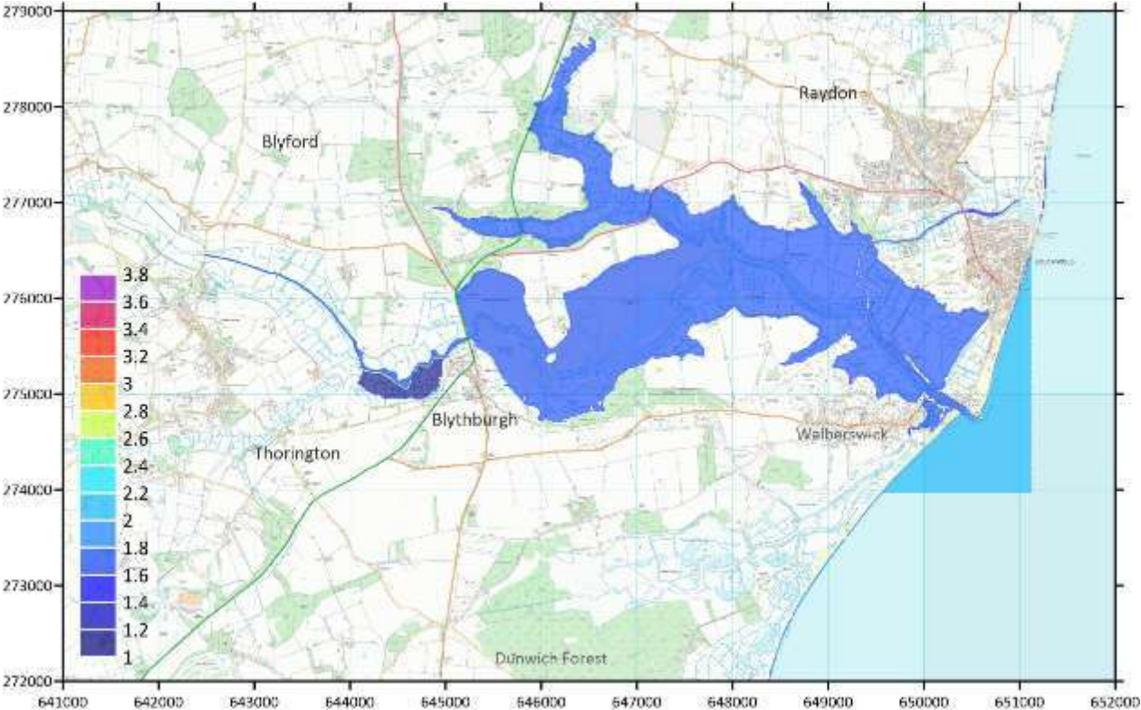
Figure 6-6: Flood extent and depth (Do Nothing, February 2020 conditions with SLR to 2070)
