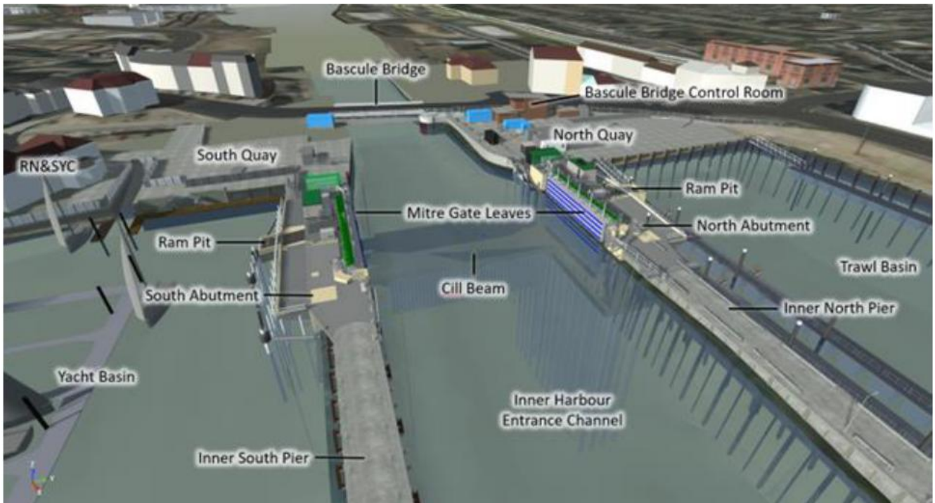
Plate 2-4: Visualisation of the proposed 40m Barrier (note: some of the plant builds to be located on the quaysides are not shown).
