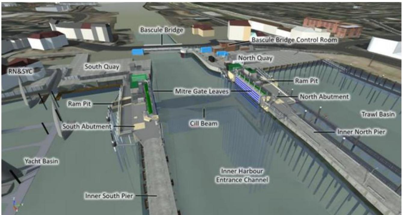
Plate 2-4: Visualisation of the proposed 40m Barrier (note: some of the plant builds to be located on the quaysides are not shown).
