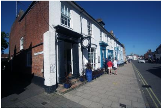
View north-east along High Street, with bitumen wearing course to the road with concrete paving slabs and concrete blocks marking some of the alley entrances, such as at Manor Farm Close.
