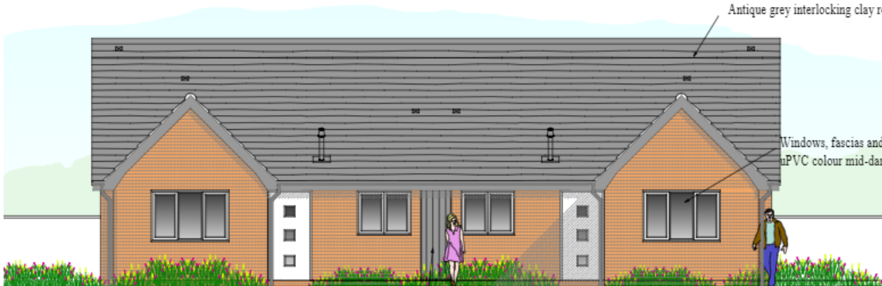
Facing bricks to be Red mottled brick with light coloured mortar FRONT ELEVATION
