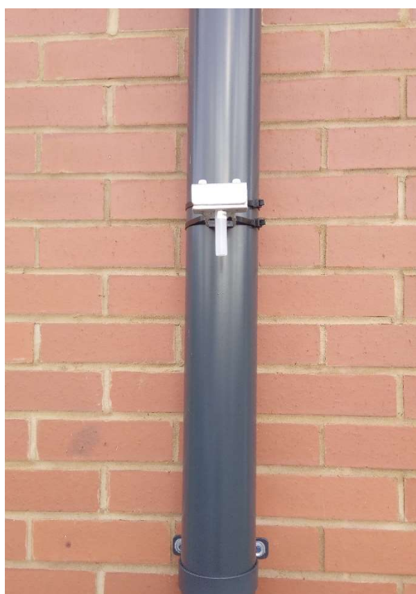
Photo 4: Diffusion tube in metal holder sited on a building’s downpipe.
