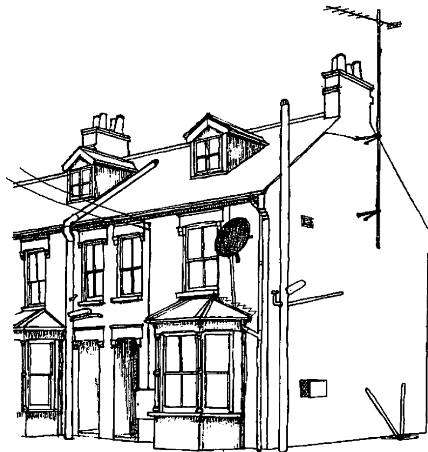
The above drawing illustrates the impact of too much external pipework
