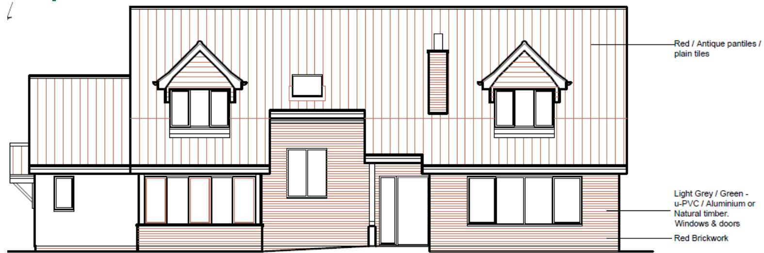
Proposed Front Elevation Scale: 1/100
