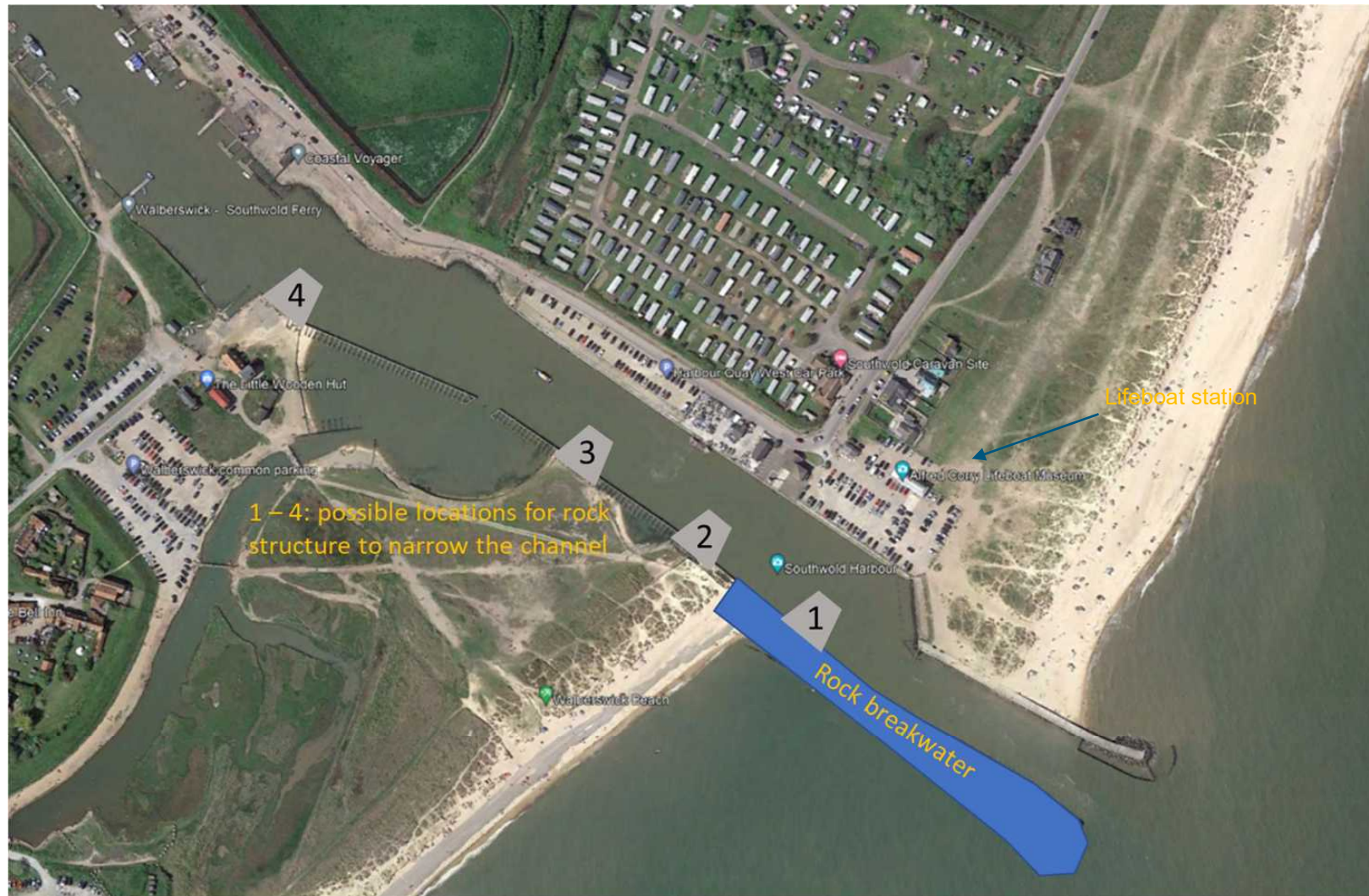
Figure 4-1: Potential locations for rock structure to extend the narrow entrance channel
