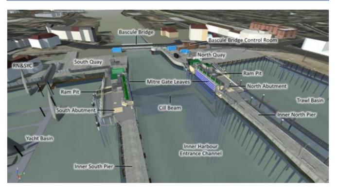
Plate 2-4: Visualisation of the proposed 40m Barrier (note: some of the plant builds to be located on the quaysides are not shown).
